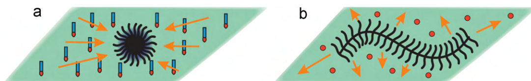
Fig. 33. Schematic of the competition in spreading between the adsorbed polymer brush molecule and co-adsorbed small molecules. (a) A co-adsorbed layer of amphiphilic molecules efficiently lowers the surface energy and causes the collapse of the macromolecules. (b) A co-adsorbed layer of polar molecules does not decrease the surface energy of the substrate and causes spreading of the macromolecules [233]. Reprinted from Gallyamov et al. by permission of the Wiley-Blackwell.
