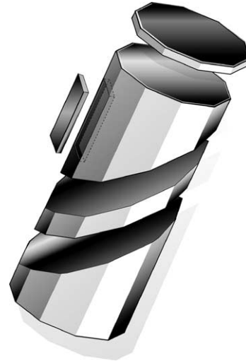
Fig. 1. Schematic drawing of a decagonal quasicrystal to illustrate orientation of samples machined for SThM and bulk thermal measurements.
