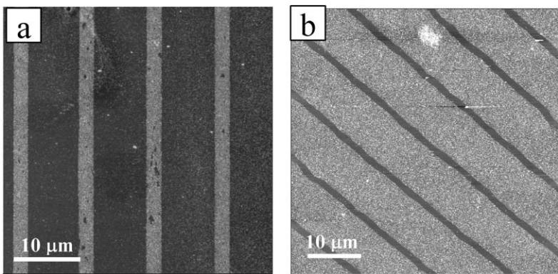
**Fig. 2** AFM images of arrays of gold nanoparticles and carbon nanotubes on the surface of polyelectrolyte multilayers, (a) gold nanoparticles (reprinted with permission from ref. 16, copyright 2005 Wiley-VCH), (b) carbon nanotubes (reprinted with permission from ref. 15, copyright 2005 The American Chemical Society).
