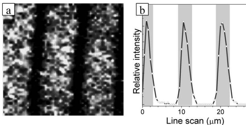
**Fig. 3** Raman scattering from nanomembranes containing Au/CNT nanostructure arrays. (a) Raman mapping of the G-line of carbon nanotube patterned nanomembranes, area  $30 \times 30 \mu\text{m}$ . Reprinted with permission from ref. 15, copyright 2005 The American Chemical Society. (b) The intensity variation of the SERS signal across several strips of the gold nanoparticle array (reprinted with permission from ref. 16, copyright 2005 Wiley-VCH).
