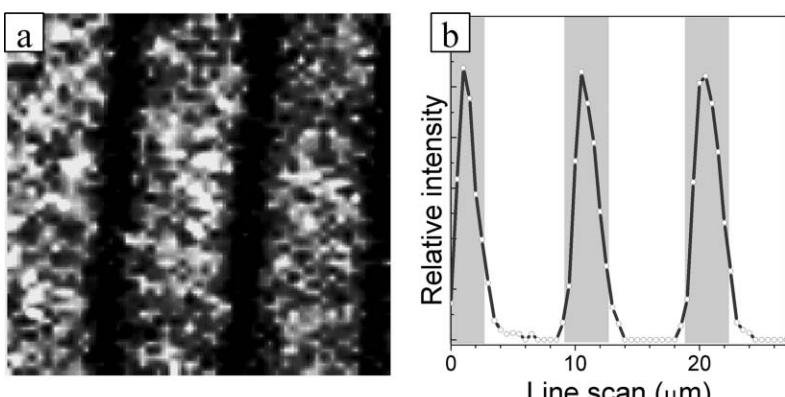
**Fig. 3** Raman scattering from nanomembranes containing Au/CNT nanostructure arrays. (a) Raman mapping of the G-line of carbon nanotube patterned nanomembranes, area  $30 \times 30 \mu\text{m}$ . Reprinted with permission from ref. 15, copyright 2005 The American Chemical Society. (b) The intensity variation of the SERS signal across several strips of the gold nanoparticle array (reprinted with permission from ref. 16, copyright 2005 Wiley-VCH).
