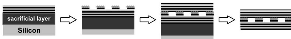
**Fig. 1** Schematic of the fabrication of a nanomembrane containing patterned arrays (not to scale).
