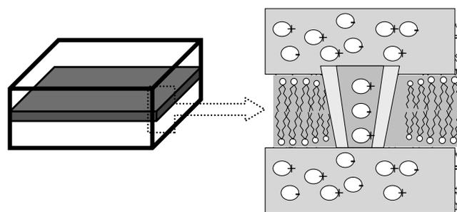
Fig. 3. The compliant interlayer with protein/lipid/hydrogel complex.
