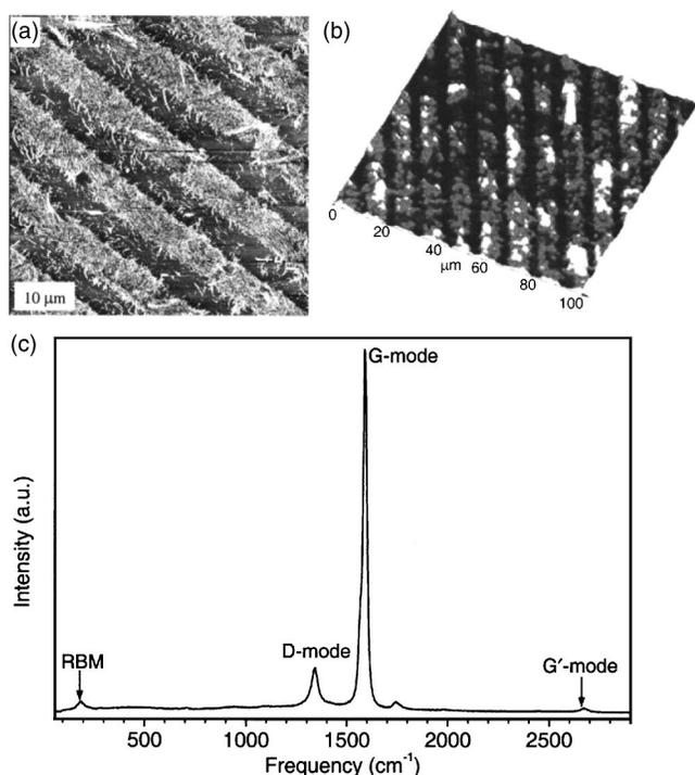
FIG. 1. (a) AFM topographical image of densely packed patterned array of carbon nanotubes. Z range is 80 nm. (b) Raman *G* mode image of patterned nanotube assembly obtained by integrating the Raman intensity at  $1590\text{ cm}^{-1}$ . The Raman intensity varies from dark (low) to bright (high). (c) Raman spectrum of patterned nanotube arrays studied, showing the RBM, the *D* mode, the *G* mode, and *G'* mode.
