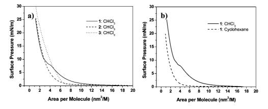
Figure 2. (a) Langmuir isotherms for 1, 2, and 3, where CHCl<sub>3</sub> was used as the spreading solvent. (b) Langmuir isotherms for 1, where cyclohexane and CHCl<sub>3</sub> were used as the spreading solvents.
