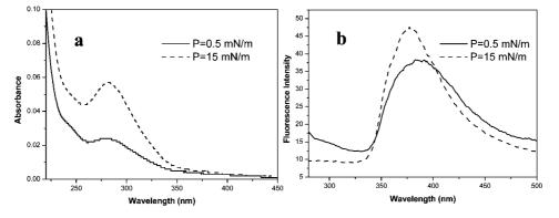
Figure 5. (a) UV-vis and (b) fluorescence spectra of 15-layer LB films of 3 deposited on quartz using the CHCl<sub>3</sub> spreading solvent.
