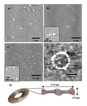
**Figure 4.** AFM topography of **3** at various surface pressures: (a) P = 0.5 mN/m, (b) P = 5 mN/m, (c) P = 10 mN/m, and (d) high-magnification image of the toroid structure at P = 0.5 mN/m. (e) A 2D schematic representation.
