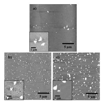
**Figure 6.** AFM topography of (a) cyclic-pressure-induced aggregation for **3** at a modest pressure of 2.5 mN/m and (b) concentration- and (c) surface-pressure-induced aggregation for **3**, both at an equivalent area per molecule at P = 20 mN/m.
