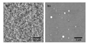
**Figure 7.** AFM topography of LB-deposited **3** at surface pressures of (a) 2 and (b) 10 mN/m using cyclohexane as the spreading solvent.
