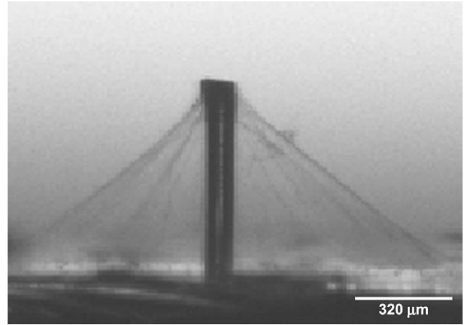
Fig. 8. Hair sensor with only small fibers attached. These fibers were spun without the use of the focusing ring where the majority of the fibers lay flat on the surface and do not form the tall structure needed for hydrogel support.
